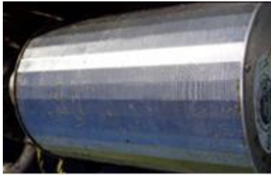
Self-cleaning screen 500 micron
