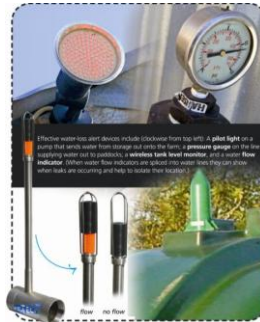
‘Alert’ system (monitored flow meter) to detect possible water loss
